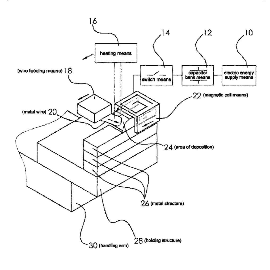
the heat source, the at least one pulsed magnetic field effecting plastic deformation of the build-up material.
