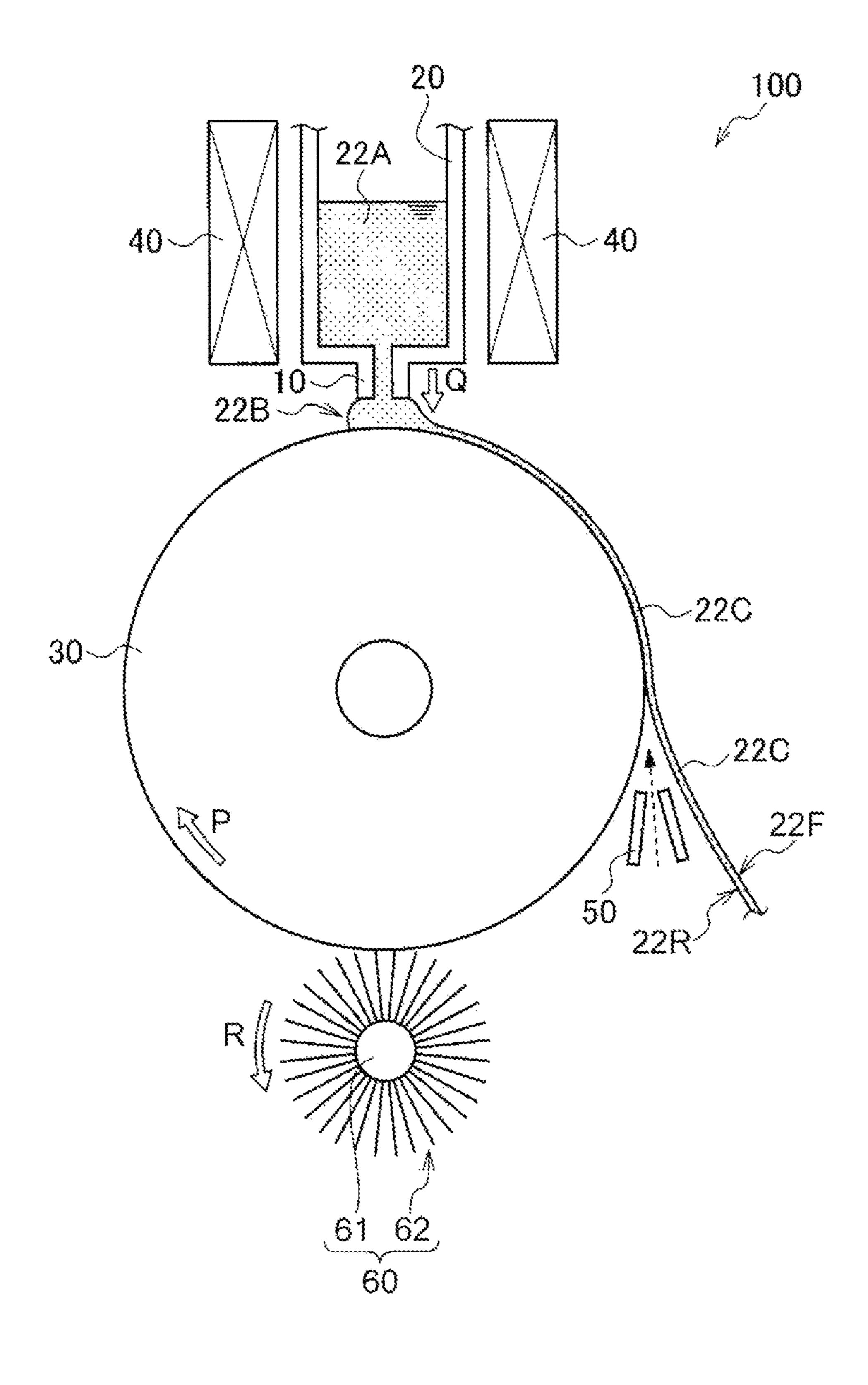
FE-BASED AMORPHOUS ALLOY RIBBON MANUFACTURING METHOD, FE-BASED AMORPHOUS ALLOY RIBBON MANUFACTURING DEVICE, AND WOUND BODY OF FE-BASED AMORPHOUS ALLOY RIBBON
