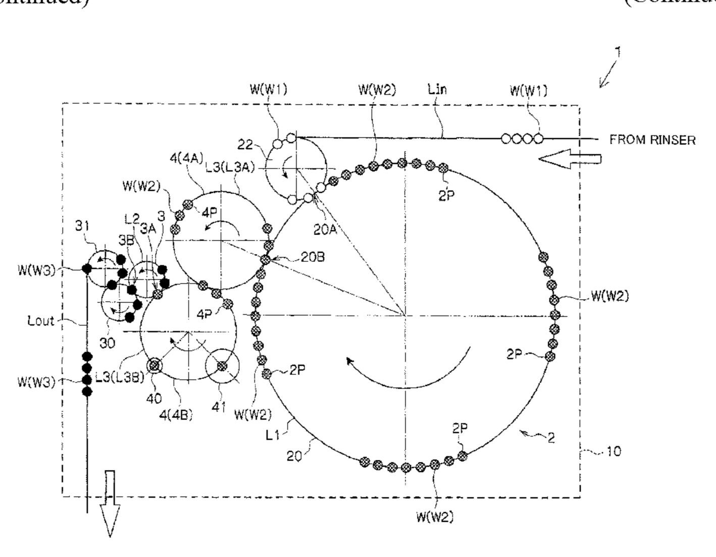
to circularly convey the can filled with the content, wherein a lid supply part is provided on the forwarding turret.
