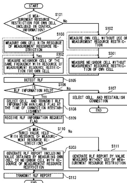
from the base station after the radio link failure occurs, the terminal generates and transmits a radio link failure report including the measurement result in the radio resources as instructed when the radio link failure occurs.
