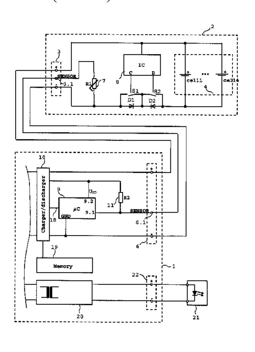
interface. The control circuit determines the type of energy storage device connected by the energy storage interface and controls the charging circuit to set the energy storage management parameter according to the determined type of energy storage device.
