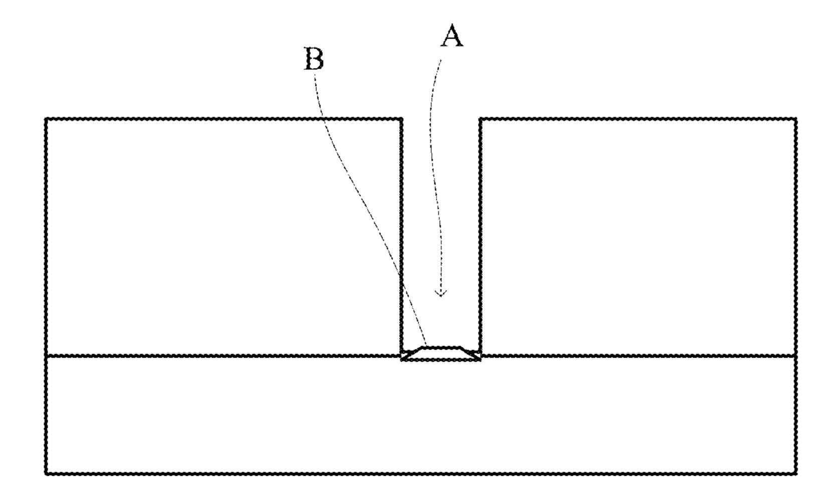
Remove a part of an object to be removed in the contact hole by a dry cleaning process <u>S31</u>
