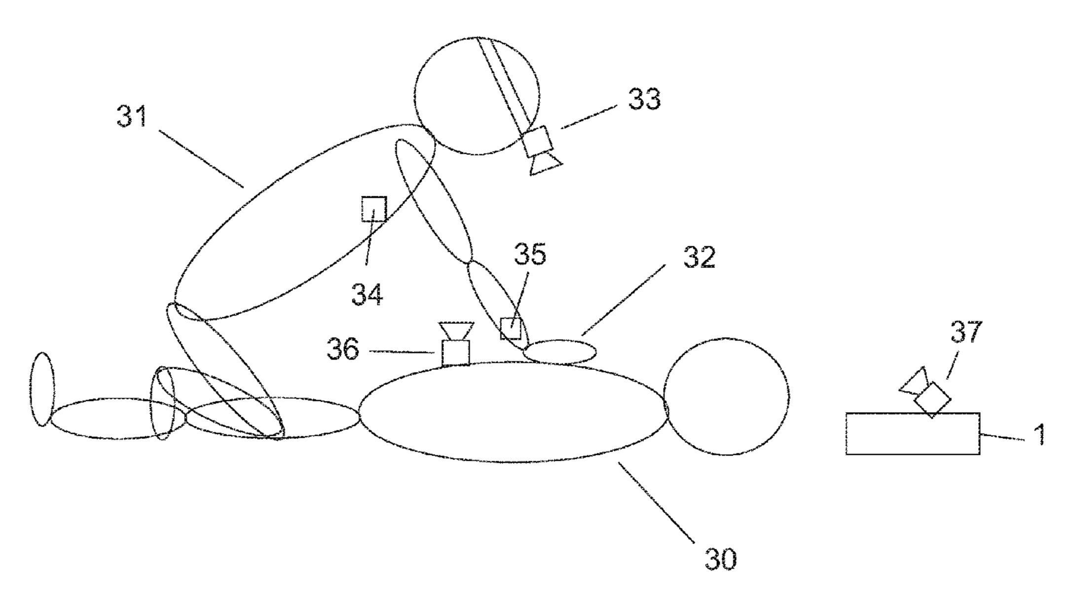
the chest compression depth and frequency can be derived from the patient facing camera by tracking the distance between the patient facing camera and the rescuer's hands.
