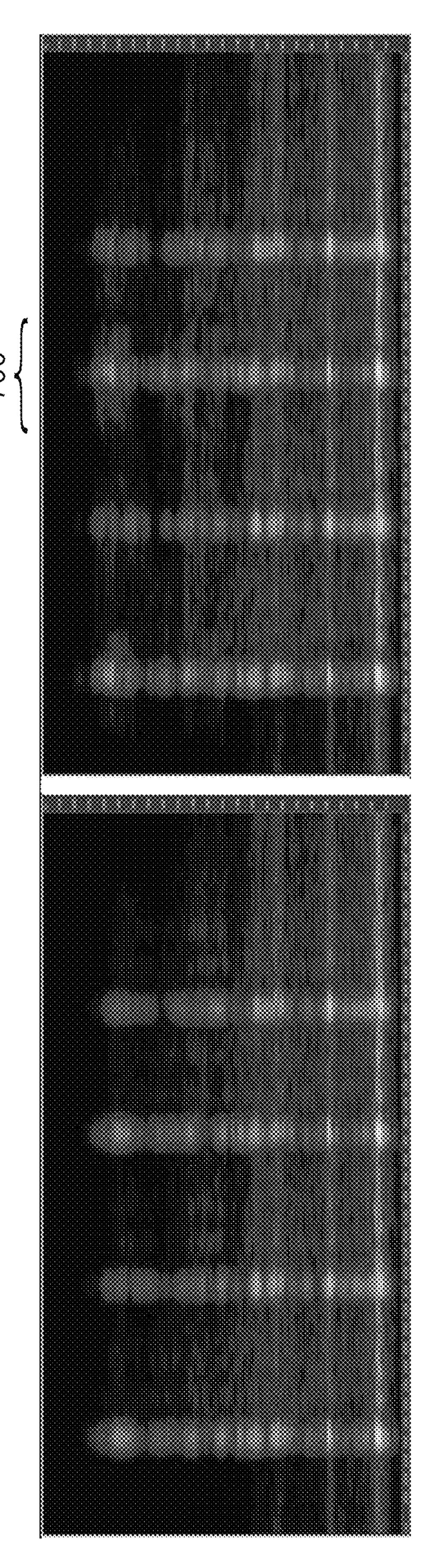
DFT spectrogram of the original signal (left panel); DFT spectrogram of the extended signal without TTS (right panel)
