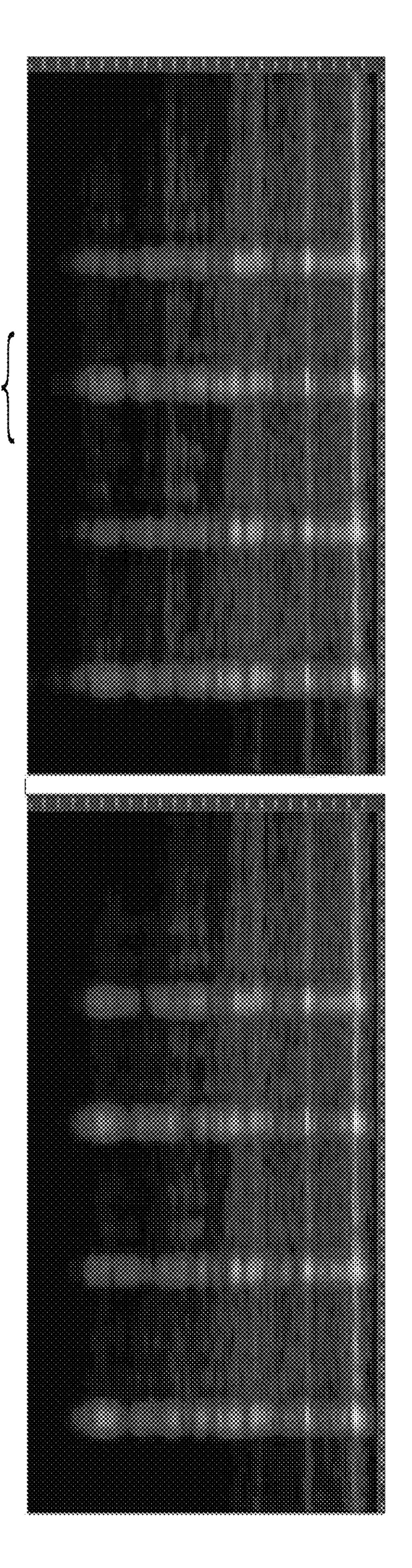
DFT spectrogram of the original signal (left panel); DFT spectrogram of the extended signal with TTS (right panel).
