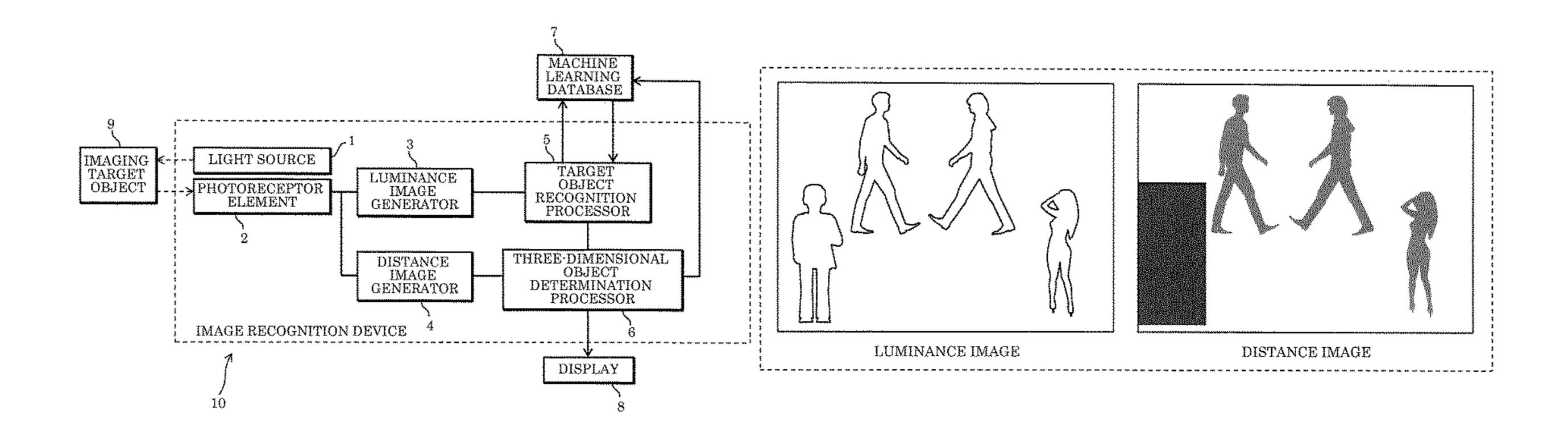
the machine learning database, as image data for extracting a feature value of a target object.
