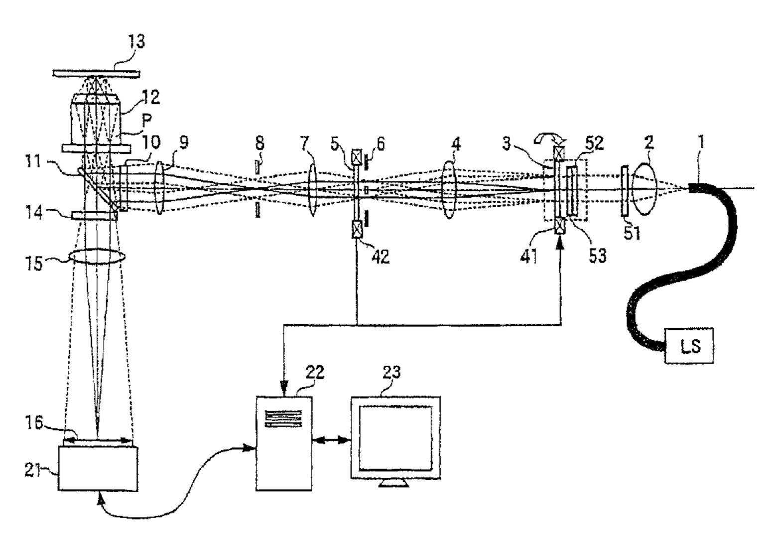
direction which allows transmitting of S polarized light. The light that has passed through the polarizer is separated into diffracted lights by a diffraction grating, and is used as the structured illumination light.
