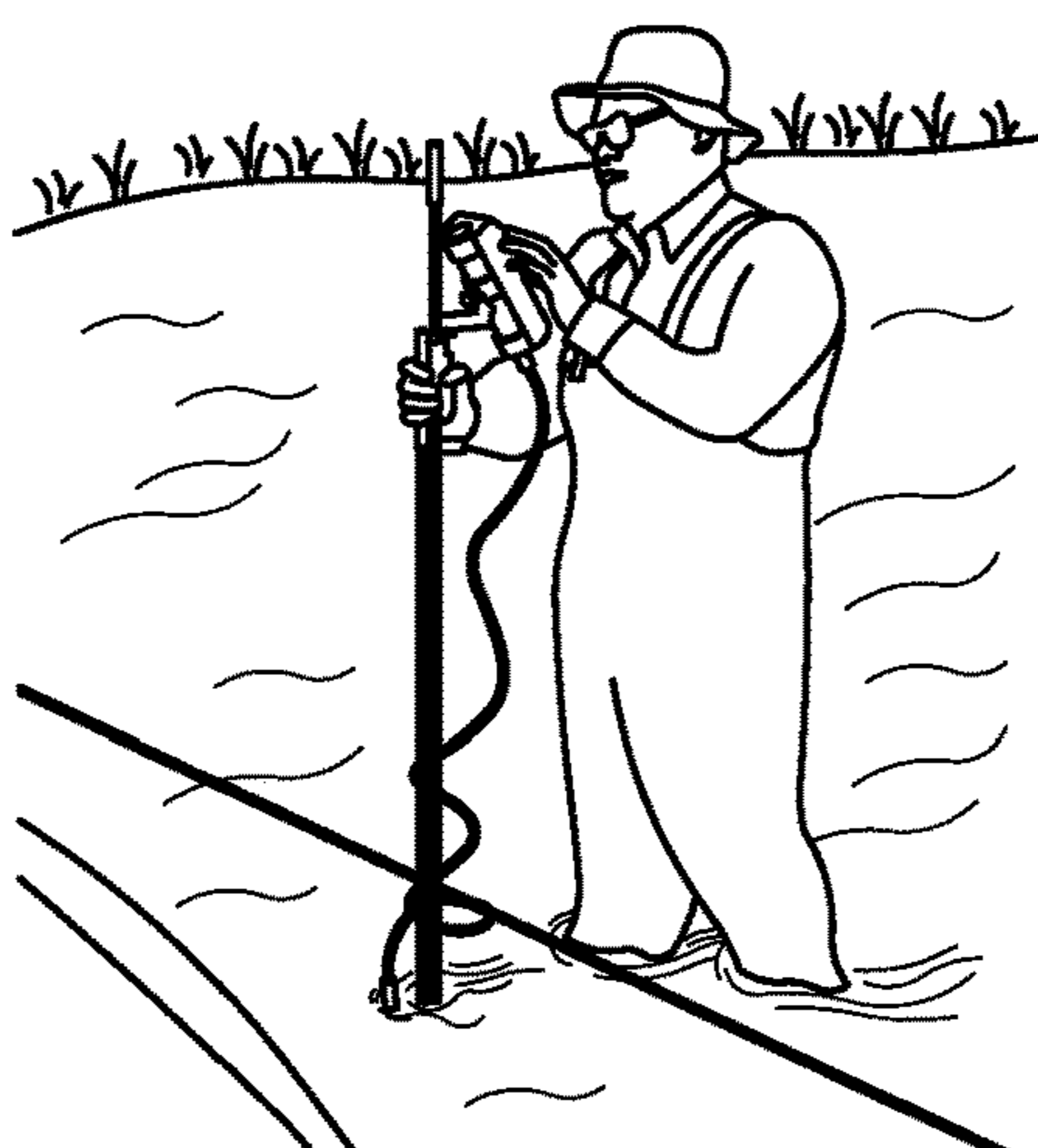
FIG. 2A: Wading Velocity Area Method (PRIOR ART)
