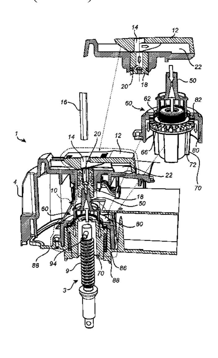
along the actuator spindle holder via the guiding arrangement. In a manual override operating mode, the actuator spindle holder is unlocked from the locking element, and the actuator spindle holder is rotatable together with the actuator spindle via the guiding arrangement.
