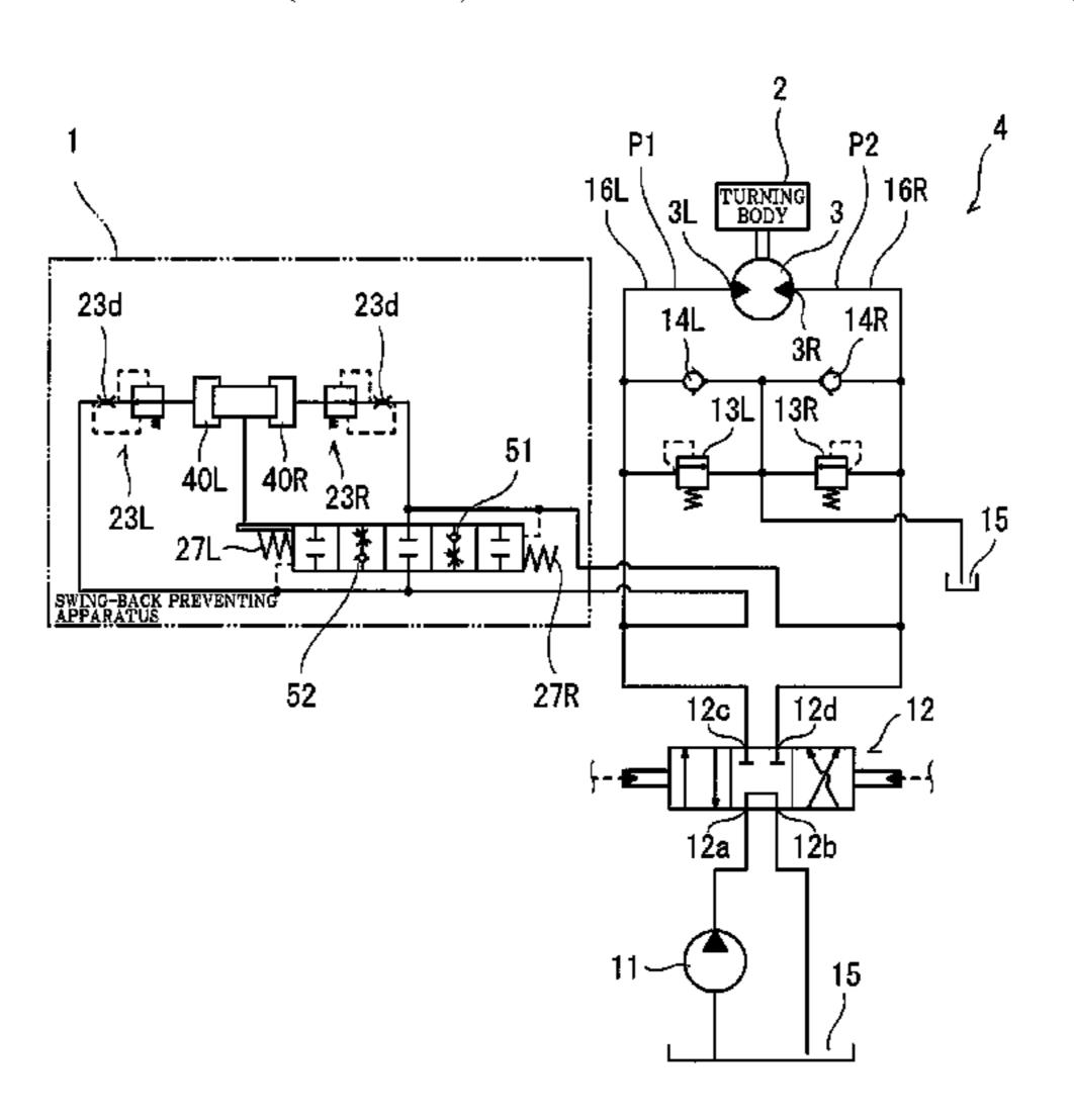
position, a second communication passage is connected to the second space. When the piston is located in a range from the neutral position to the first offset position, the second communication passage is blocked from the second space.
