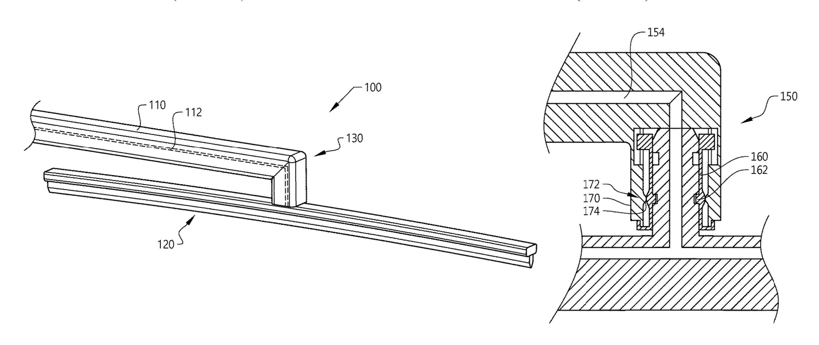
wherein said wall (170) comprises a constricted section (172) whereby an inner wall (174) of said constricted section (172) is configured to press the radial protrusion (162) radially inwards when the constricted section (172) is axially aligned with the radial protrusion (162).
