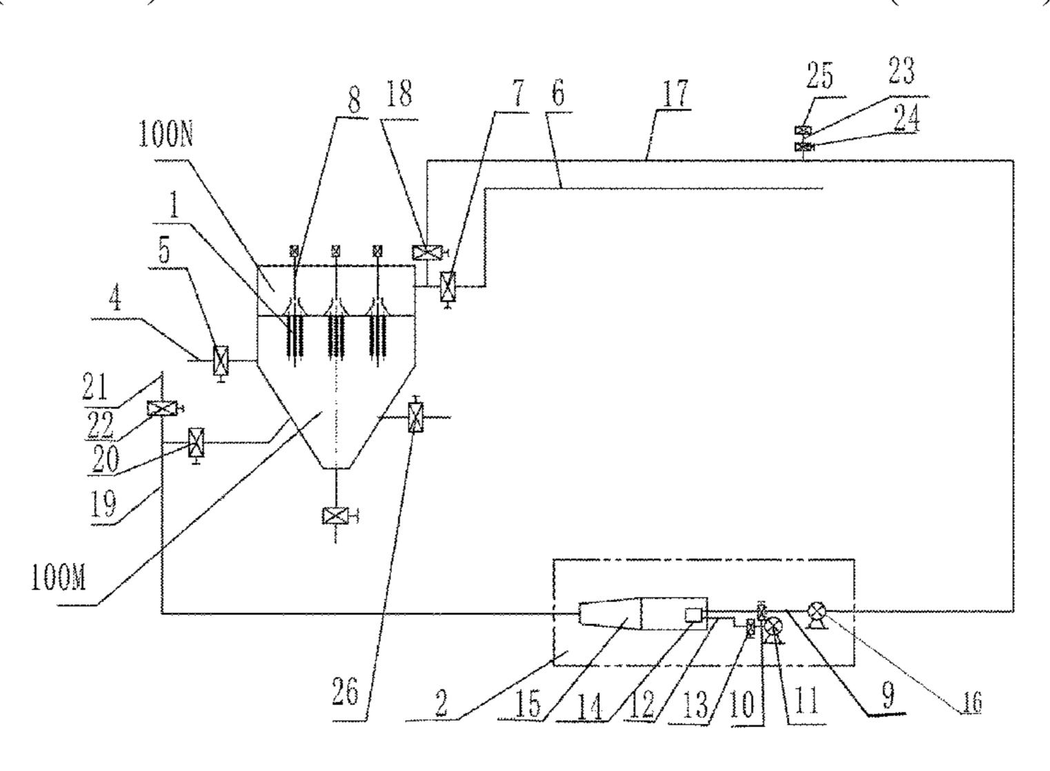
filtering devices and a pre-heating apparatus and regeneration apparatus provided for the high-temperature dust removal and filtering devices. Said method is implemented with a high-temperature dust removal and filtering system capable of switching. The high-temperature dust removal and filtering system always keeps one or more sets of high-temperature dust removal and filtering devices in a normal filtering state.
