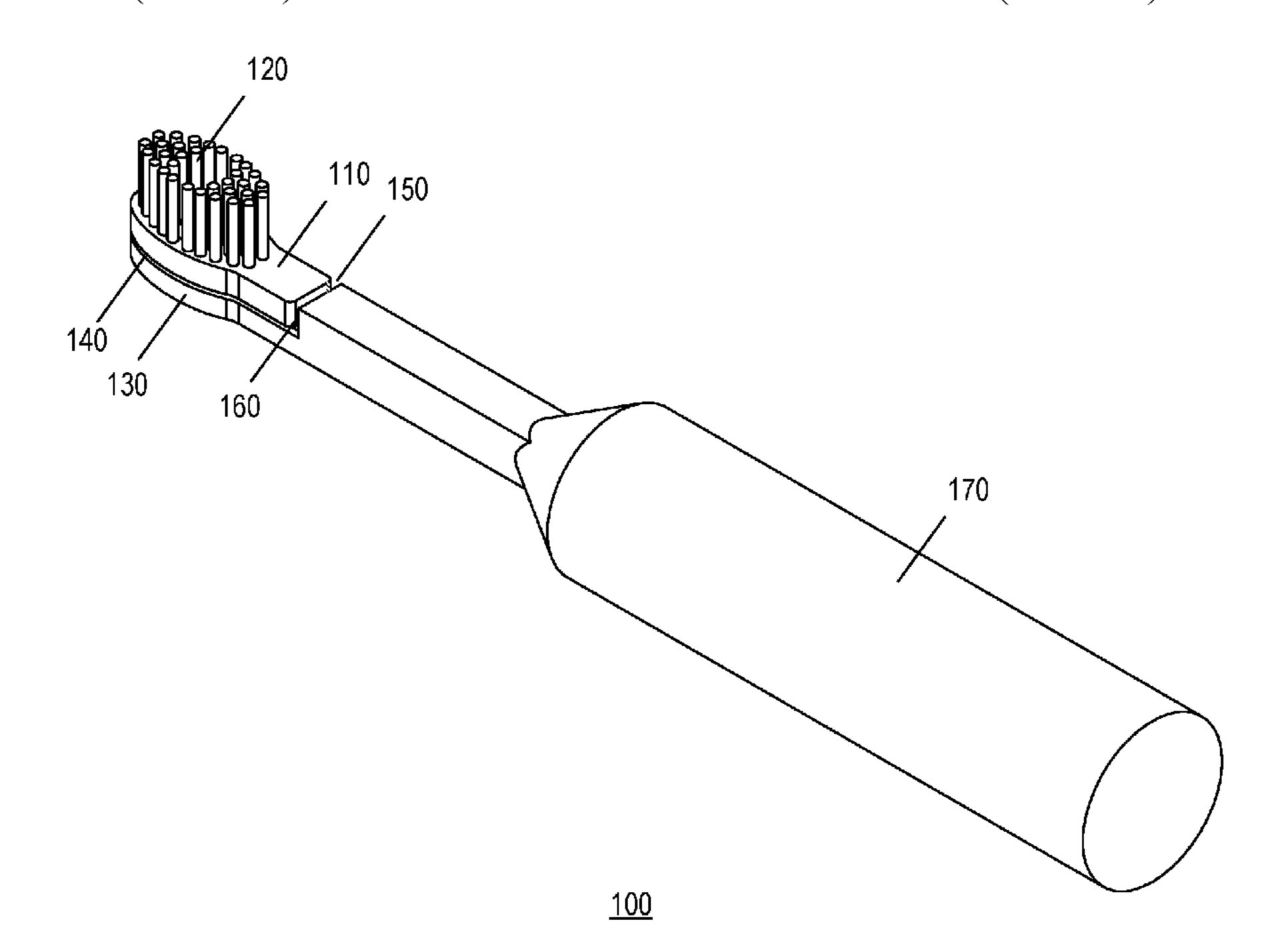
bristles projecting in a first direction. The cleaning head may define a central opening. The central opening may be arranged to provide the camera with a view in the first direction.
