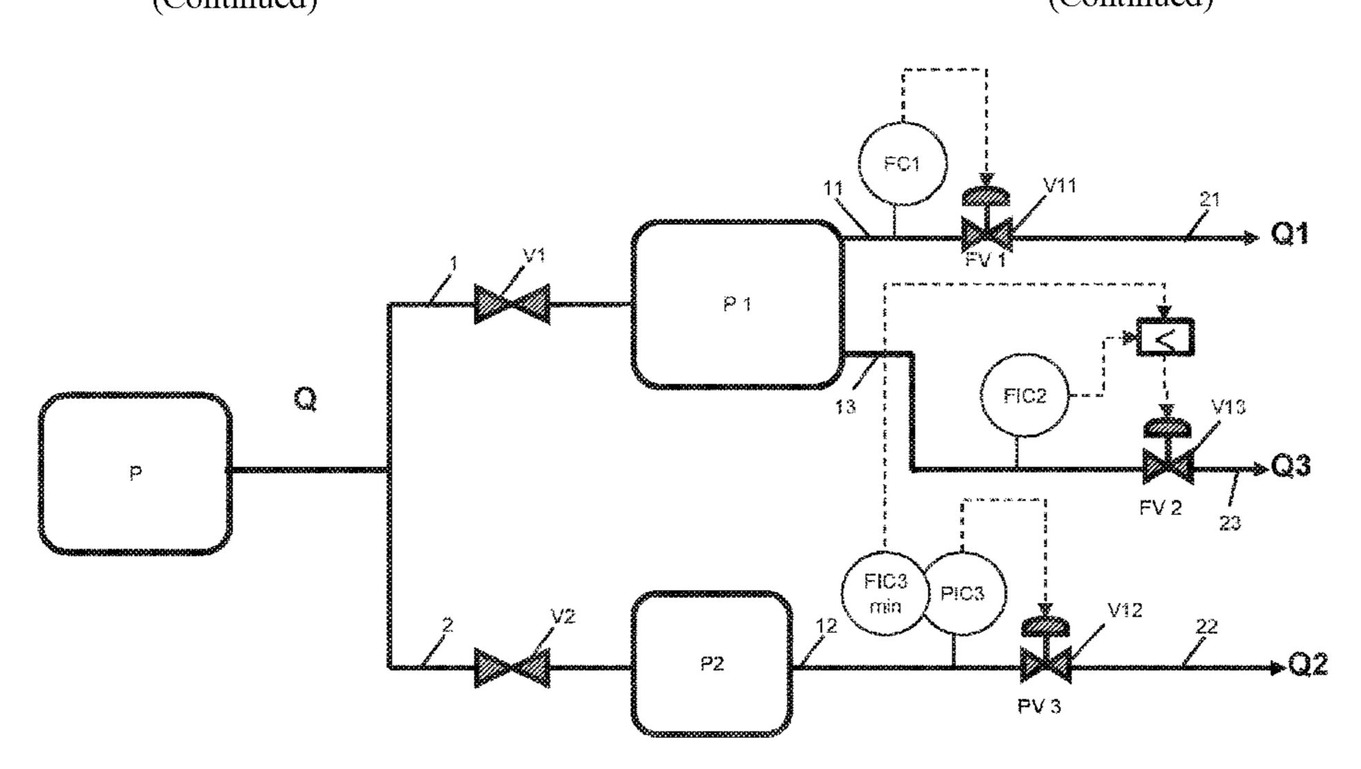
processed flow having a value Q1 in nominal operation is reduced to a value less than Q1.
