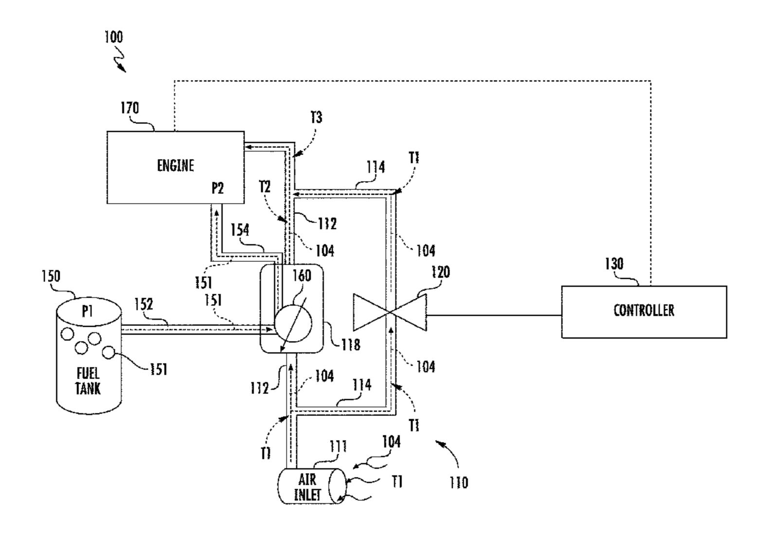
configured to adjust the air flowing through at least one of the first air supply line and the second air supply line.
