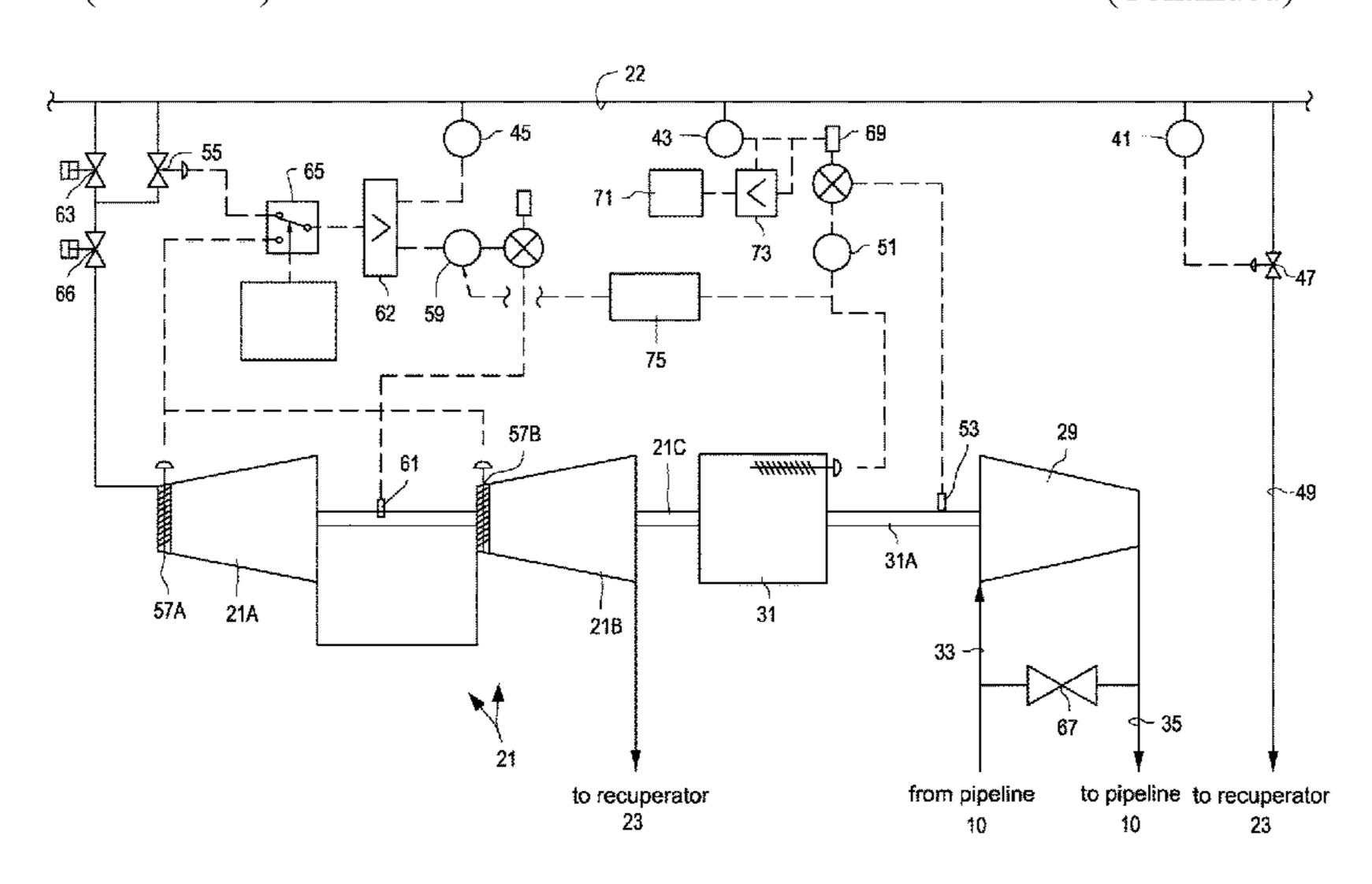
variable-speed mechanical coupling between the turboexpander and the rotating load.
