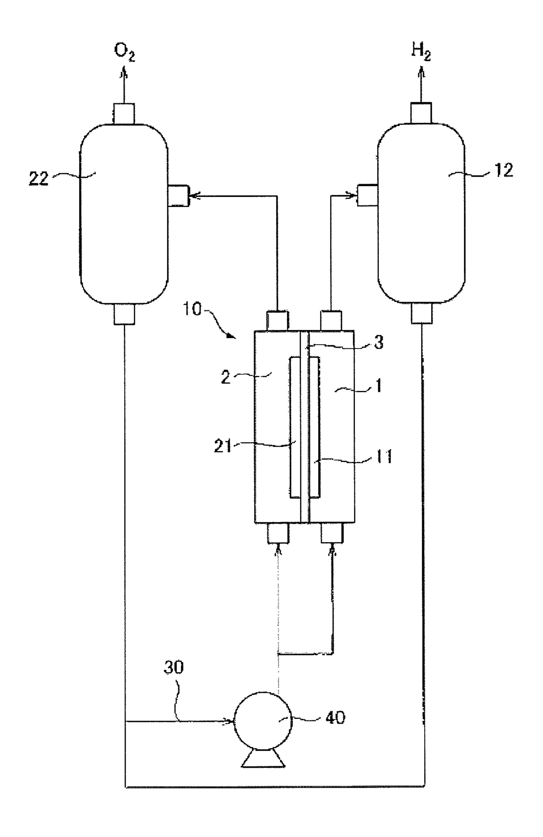
DIAPHRAGM FOR ALKALINE WATER ELECTROLYSIS, ALKALINE WATER ELECTROLYSIS DEVICE, METHOD FOR PRODUCING HYDROGEN, AND METHOD FOR PRODUCING DIAPHRAGM FOR ALKALINE WATER ELECTROLYSIS
