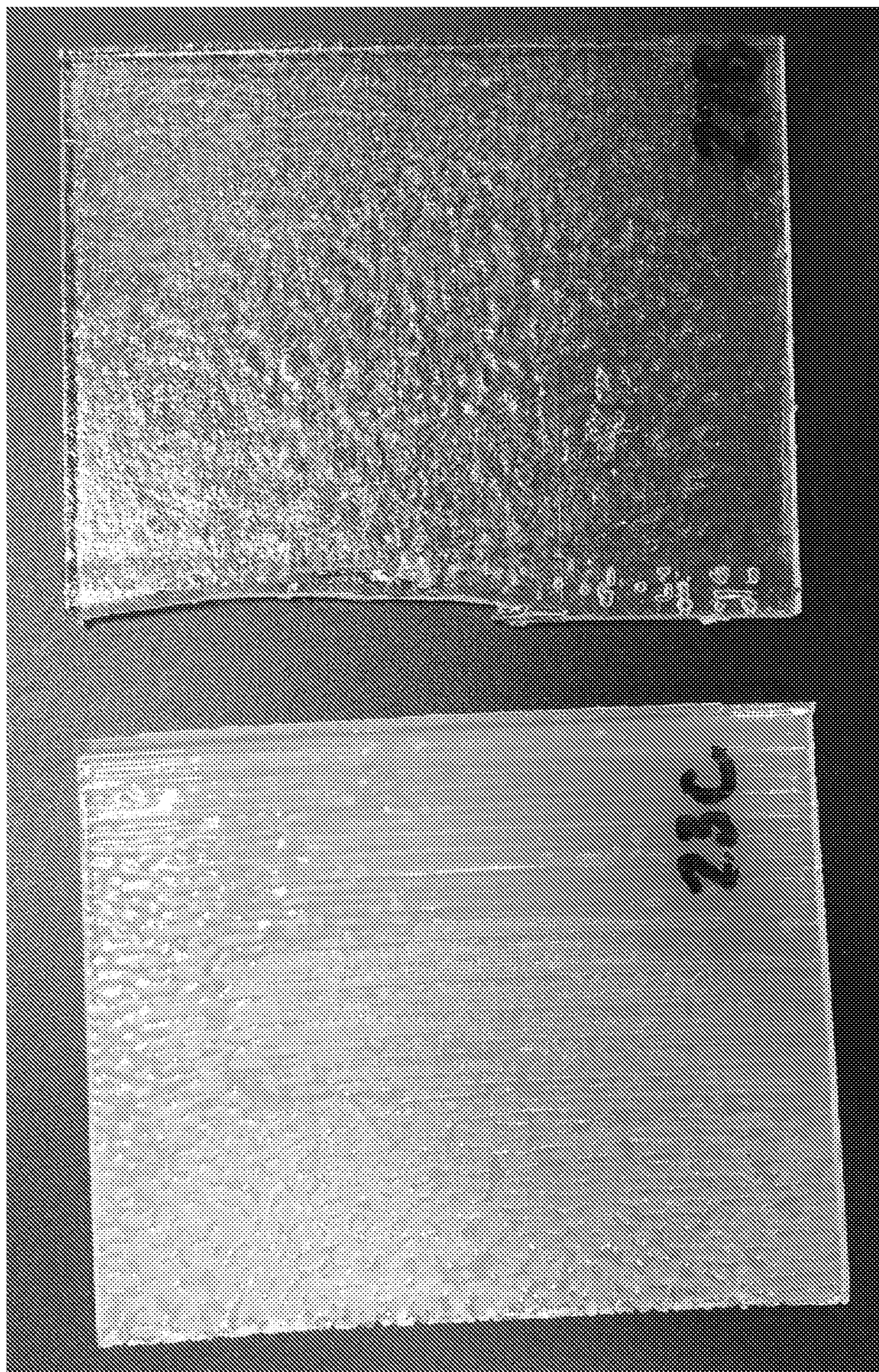
Figure 3: Polyether amine hardener system Without CN153 (left); with CN153 (right)
