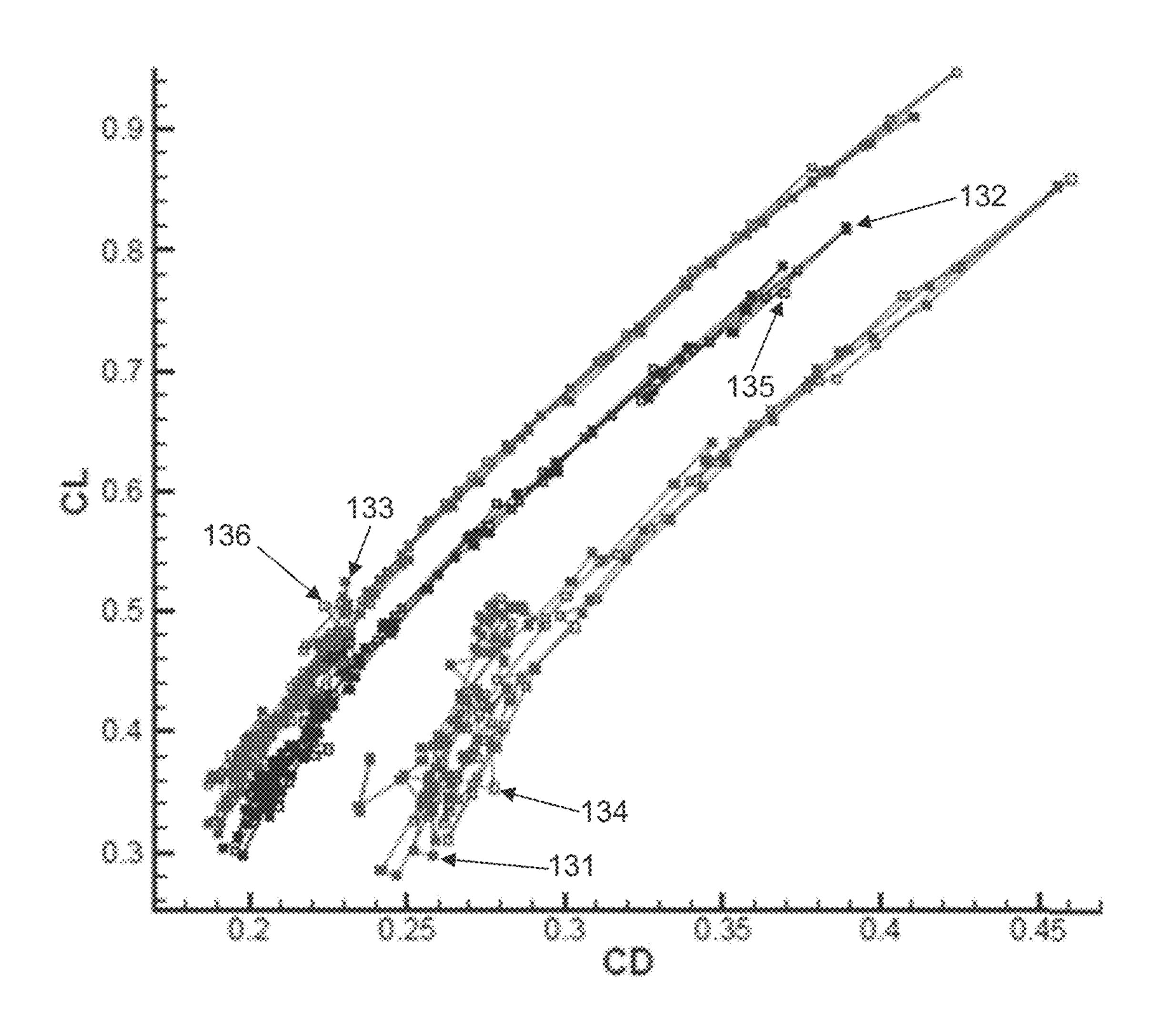
(131) Re = 40k: LE=20° TE= 0° to 20° to -20° to 0° (132) Re = 80k: LE=20° TE= 0° to 20° to -20° to 0° (133) Re = 160k: LE=20° TE= 0° to 20° to -20° to 0° (134) Re = 40k: LE=20° TE= 0° to -20° to 20° to 0° (135) Re = 80k: LE=20° TE= 0° to -20° to 20° to 0° (136) Re = 1600k: LE=20° TE= 0° to -20° to 20° to 0°
