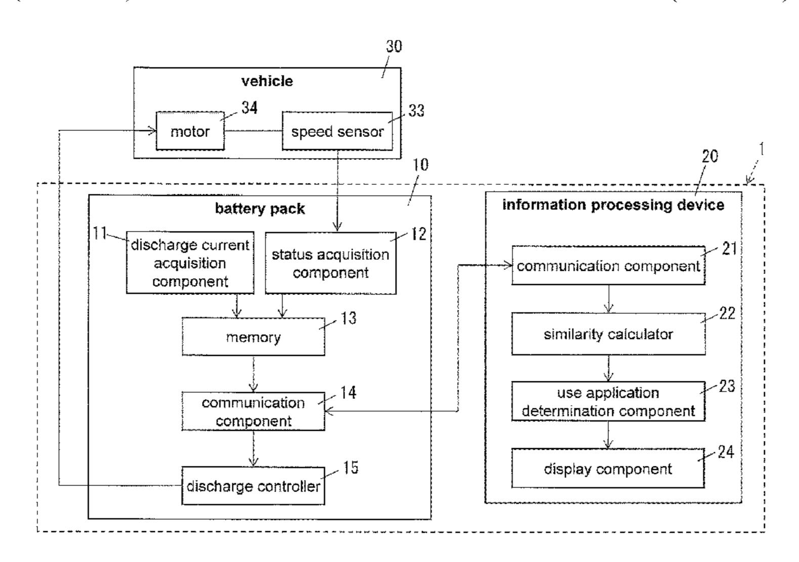
whether or not the battery pack is being used for something other than its intended use application, according to the similarity calculated by the similarity calculator (112).
