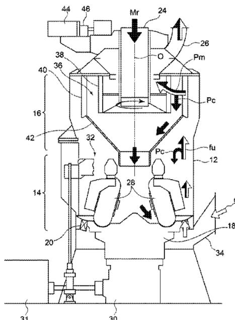
annular flow passage between the inner ring and the outer ring; and a plurality of throat vanes disposed between the inner ring and the outer ring. The following expressions are satisfied:  $2.0 \leq L/d \leq 4.0$ ; and  $0.5 \leq H/d \leq 1.5$ , where H is a gap between the inner ring and the outer ring with respect to a radial direction, L is a length of the throat vanes, and 'd' is a distance between adjacent two of the throat vanes.
