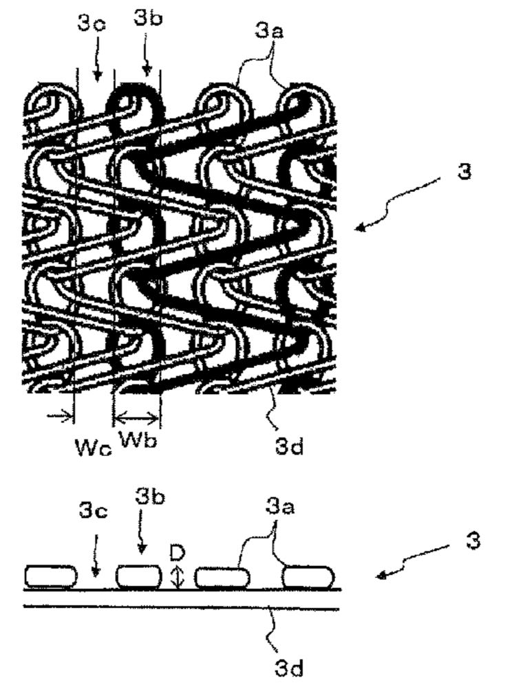
flow-channel member comprises a tricot knitted fabric having a plurality of ribs each formed by repeating loops in a linear form in a longitudinal direction, and a plurality of grooves present between the ribs; has a membrane support index of 60 to 135, the membrane support index being calculated in accordance with the specified numerical relationship.
