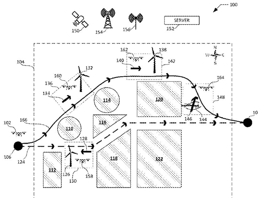
the drone to be at least partially propelled by wind to reduce energy consumed by the drone during the flight.
