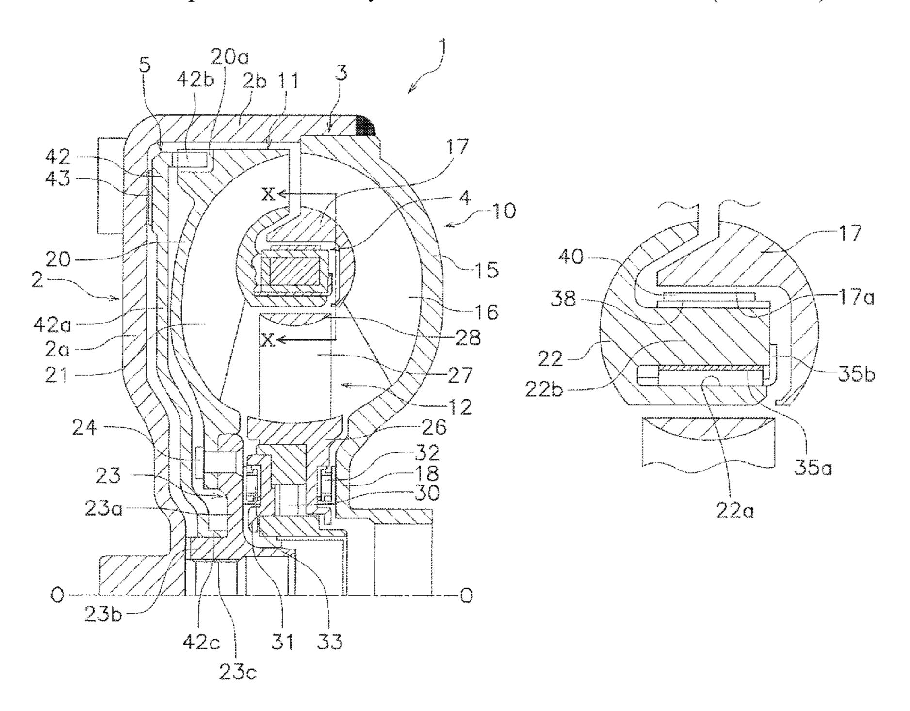
trifugal clutch is disposed in a space between the impeller core and the turbine core. The centrifugal clutch is configured to directly transmit the power from the impeller to the turbine when a rotational speed of the turbine is greater than or equal to a predetermined value.
