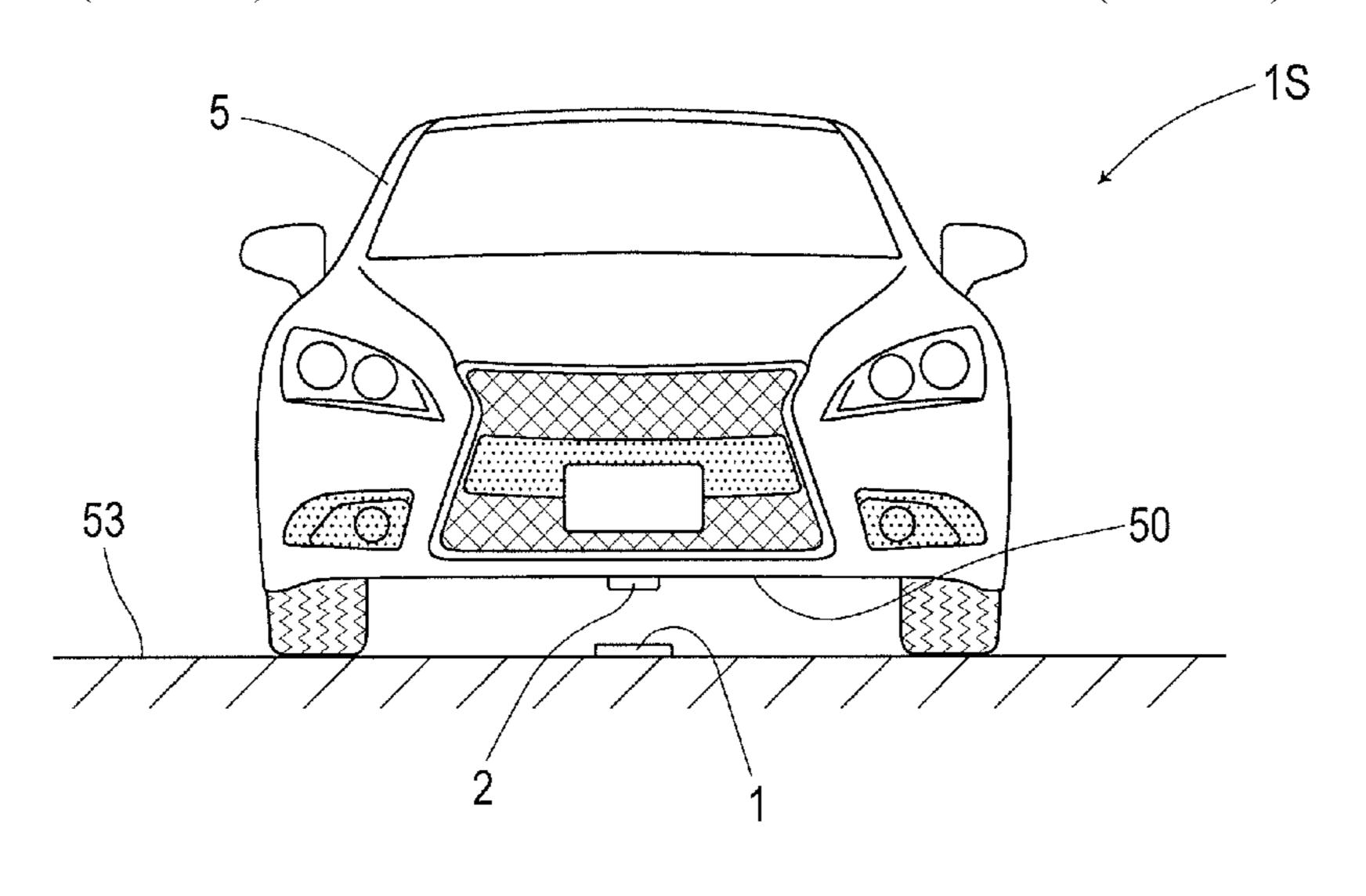
combination, the magnetic marker having a surface with a magnetic flux density equal to or smaller than 40 mT and the magnetic sensor using a magneto-impedance element including an amorphous wire as a magneto-sensitive body with impedance in a high-frequency region changing in accordance with an external magnetic field.
