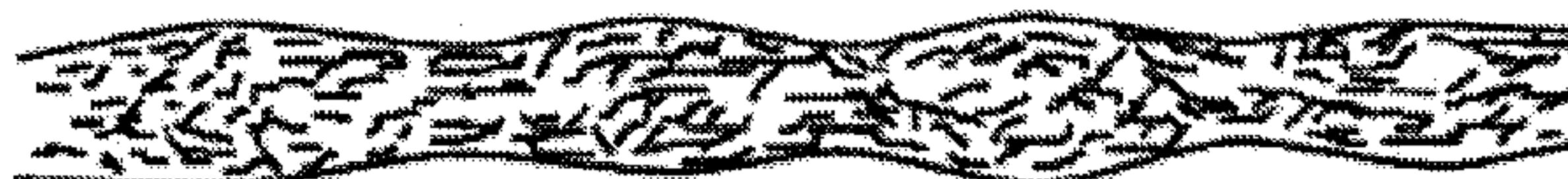
Air Rich yarn --" homogeneous porous structure"
