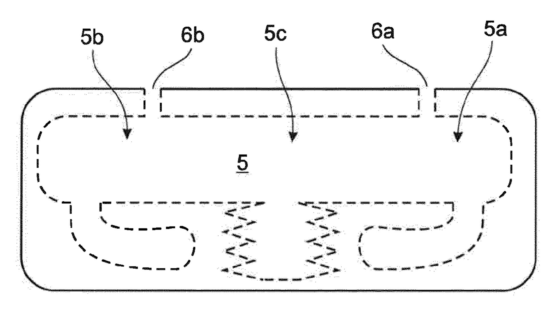
mounted to a vehicle seat, limit the lateral movement of the torso of an occupant and protect an occupant. The third portion will contribute with an increased stability of the air bag device when deployed. The air bag device may be adapted to protect the head of an occupant from injuries.
