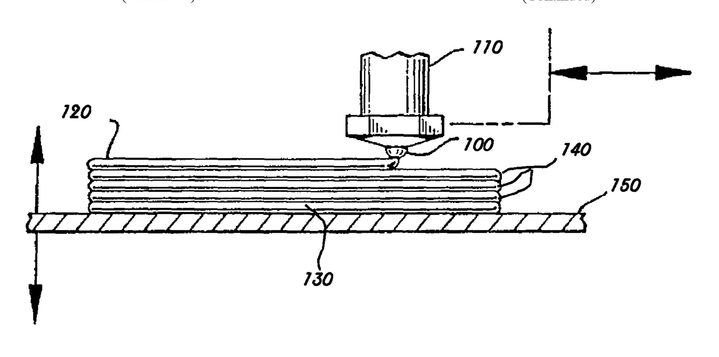
surface flow of material into valleys between the extrudates as they are being built up.
