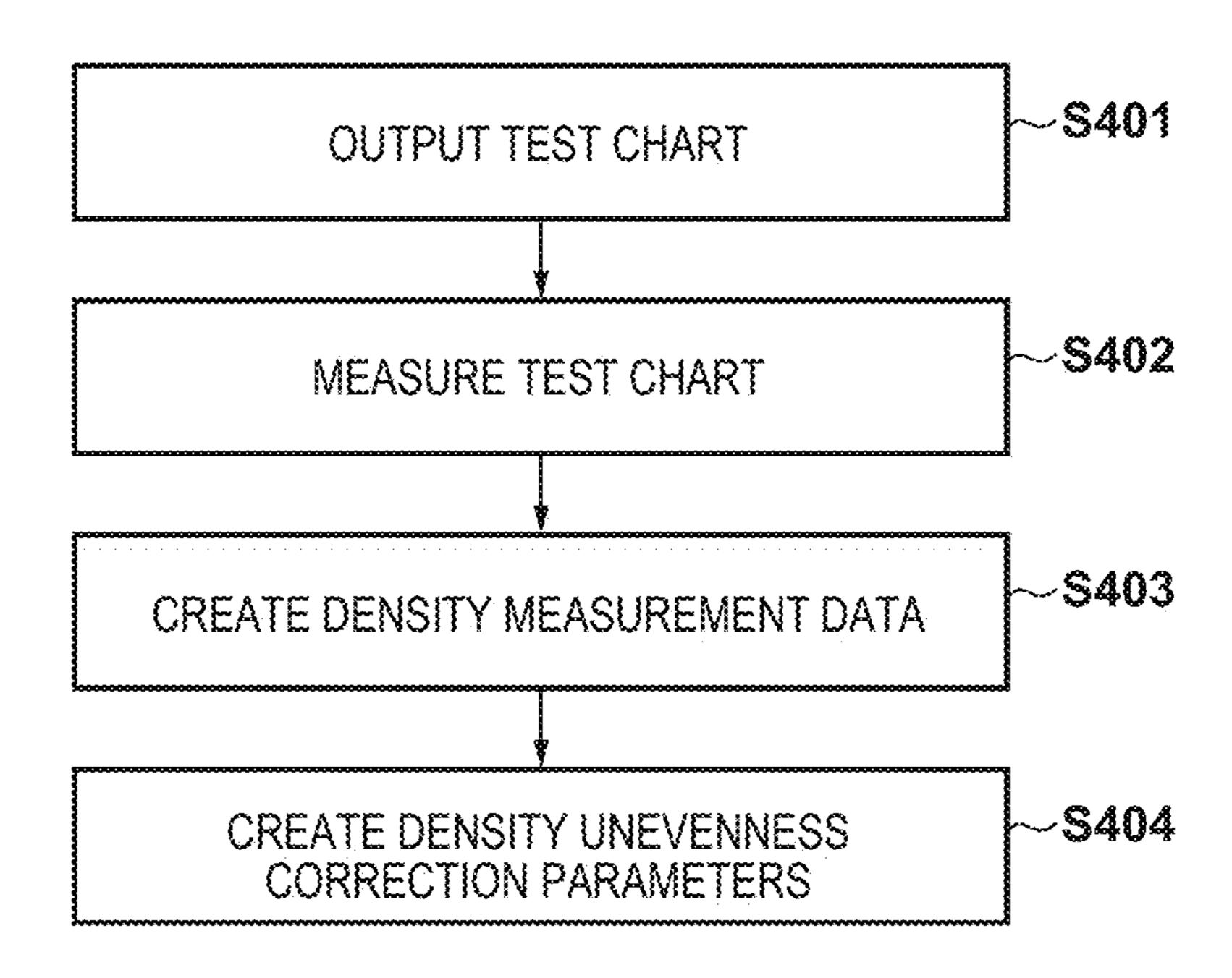
IMAGE PROCESSING APPARATUS, CONTROL METHOD THEREOF, AND NON-TRANSITORY COMPUTER-READABLE STORAGE MEDIUM THAT EXECUTE A DENSITY UNEVENNESS CORRECTION PROCESS IN ACCORDANCE WITH PROPERTIES OF RECORDING ELEMENTS
