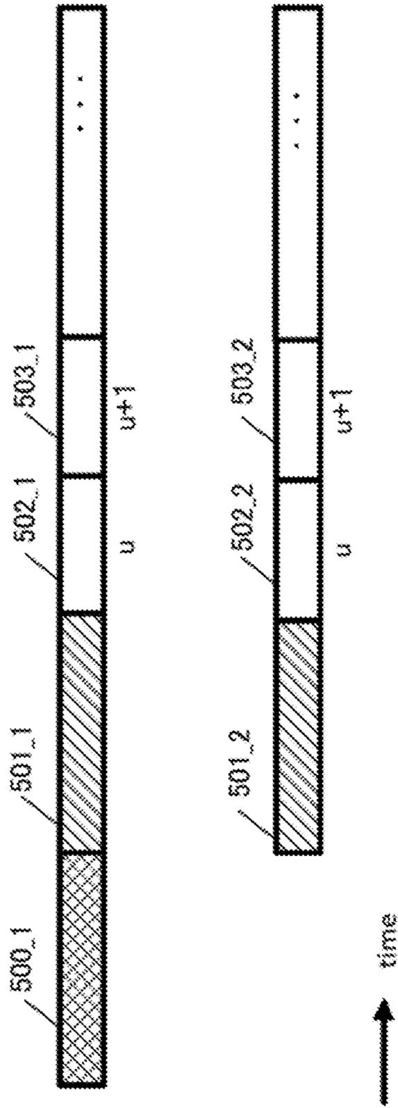
Modulated signal  $z_1(t)$  frame configuration
