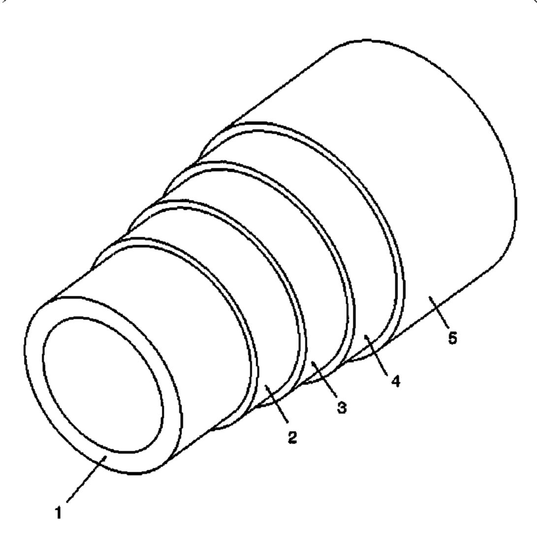
additionally has the step of optionally winding a perforated layer on top of an outermost layer of the layers of woven fabric to remove excess resin when the woven fabric is wound over the composite sleeve. The method also includes the steps of wrapping an absorption layer over the composite sleeve for absorbing the excess resin, curing the thermoset resin, and removing the absorption layer and the perforated layer after the curing.
