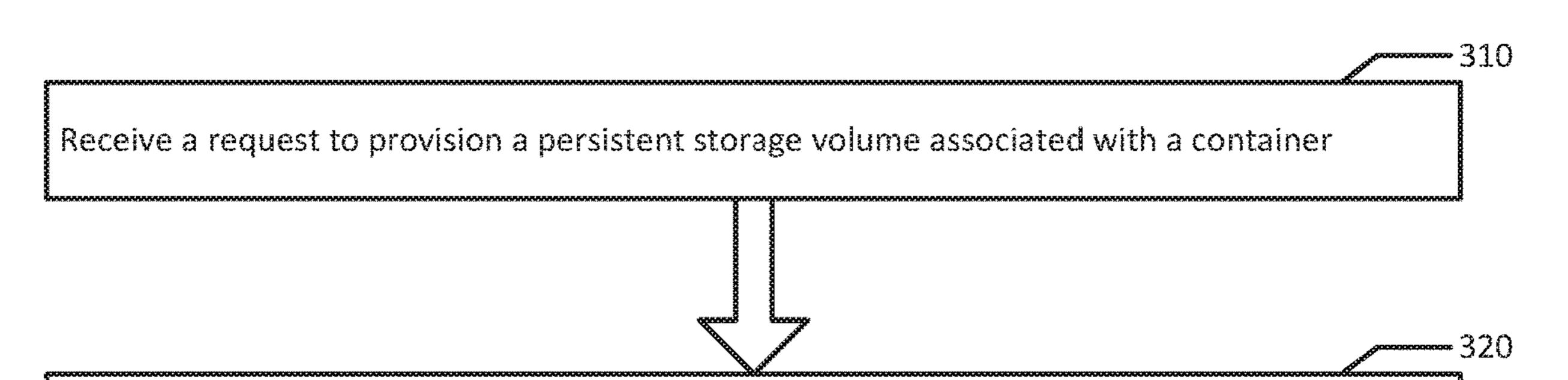
Create the persistent storage volume in a storage pool based on a storage mode stored in metadata associated with the container that includes a deduplication mode, a compression mode, and/or an encryption mode
