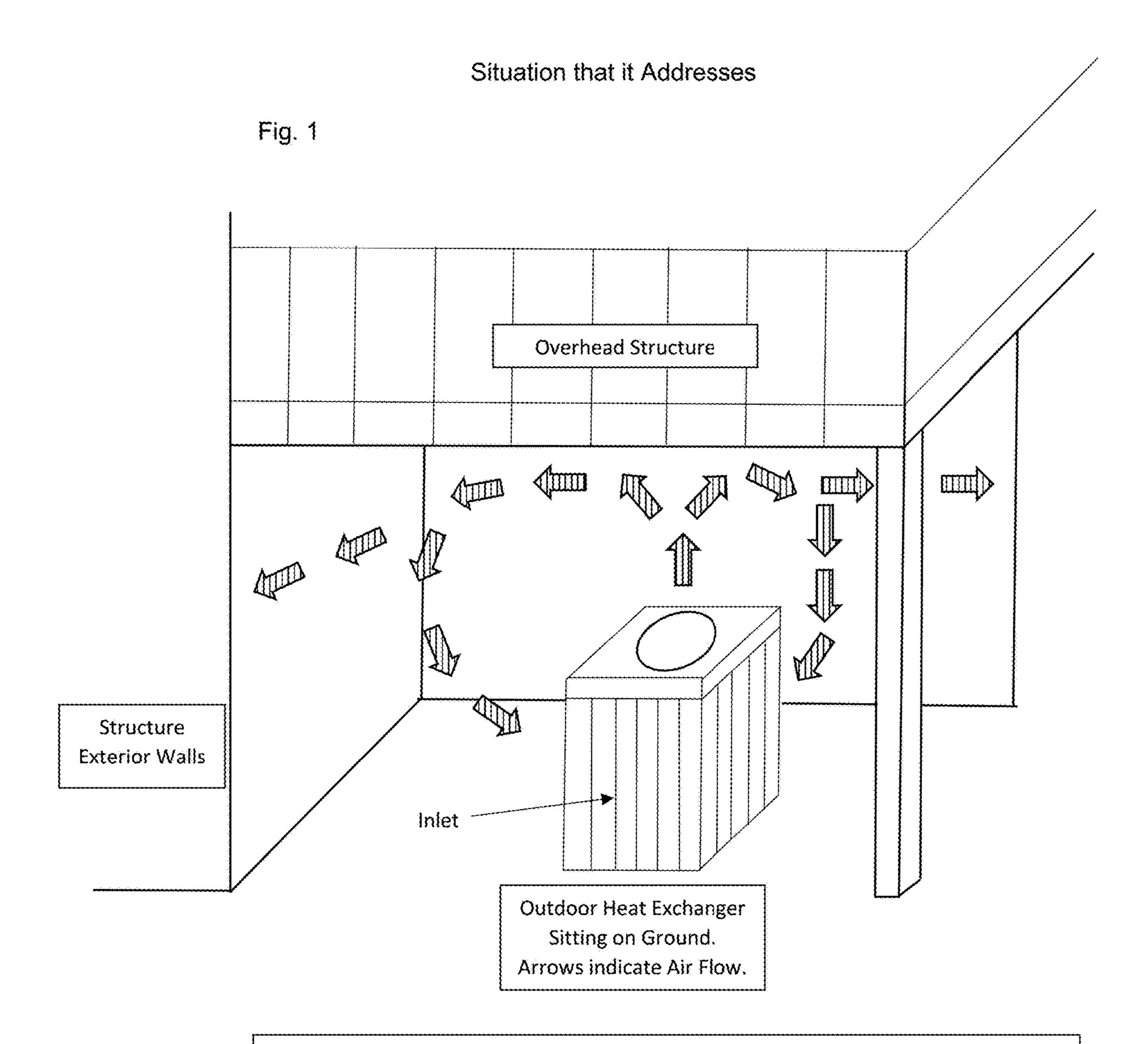
Explanation: This is the situation before the invention is installed. The nearby structure and overhead structure cause a percentage of upward discharge air to recirculate to the inlet. This is confirmed by actual temperature measurement. Inlets are on all four faces of the Exchanger.
