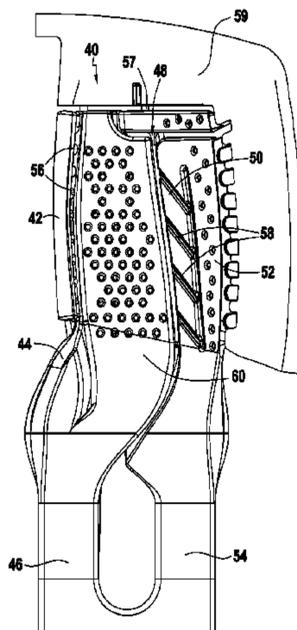
to a core portion that is to form at least one central cavity, firstly in the core root via at least two ceramic junctions, and secondly at various heights up the core via a plurality of other ceramic junctions of positioning that defines the thickness of the internal partitions of the blade, while also ensuring additional cooling air for predetermined critical zones of the first and second lateral cavities.
