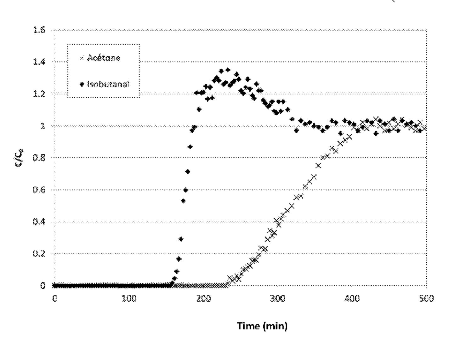
simultaneously eliminating the isobutanal and the acetone being carried out at a temperature of between 0 and 200° C., at a pressure of 0.1 to 10 MPa and with an hourly space velocity of the feedstock over the fixed bed of 0.1 to 10 h<sup>-1</sup>.
