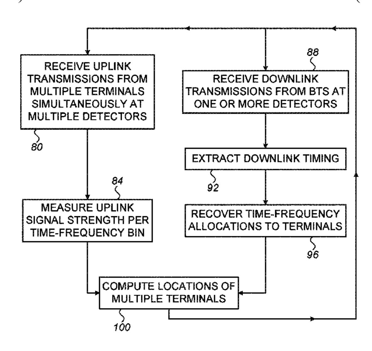
system is able to distinguish between the uplink signal components originating from each terminal, and thus compute the location of each terminal.
