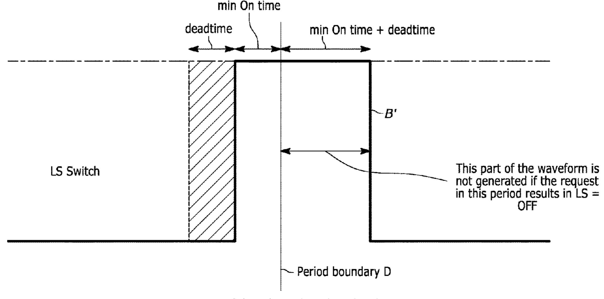
Any requested duty that is less than the above diagram which yields LS On time before deadtime insertion = 2\*(deadtime + min On time)
