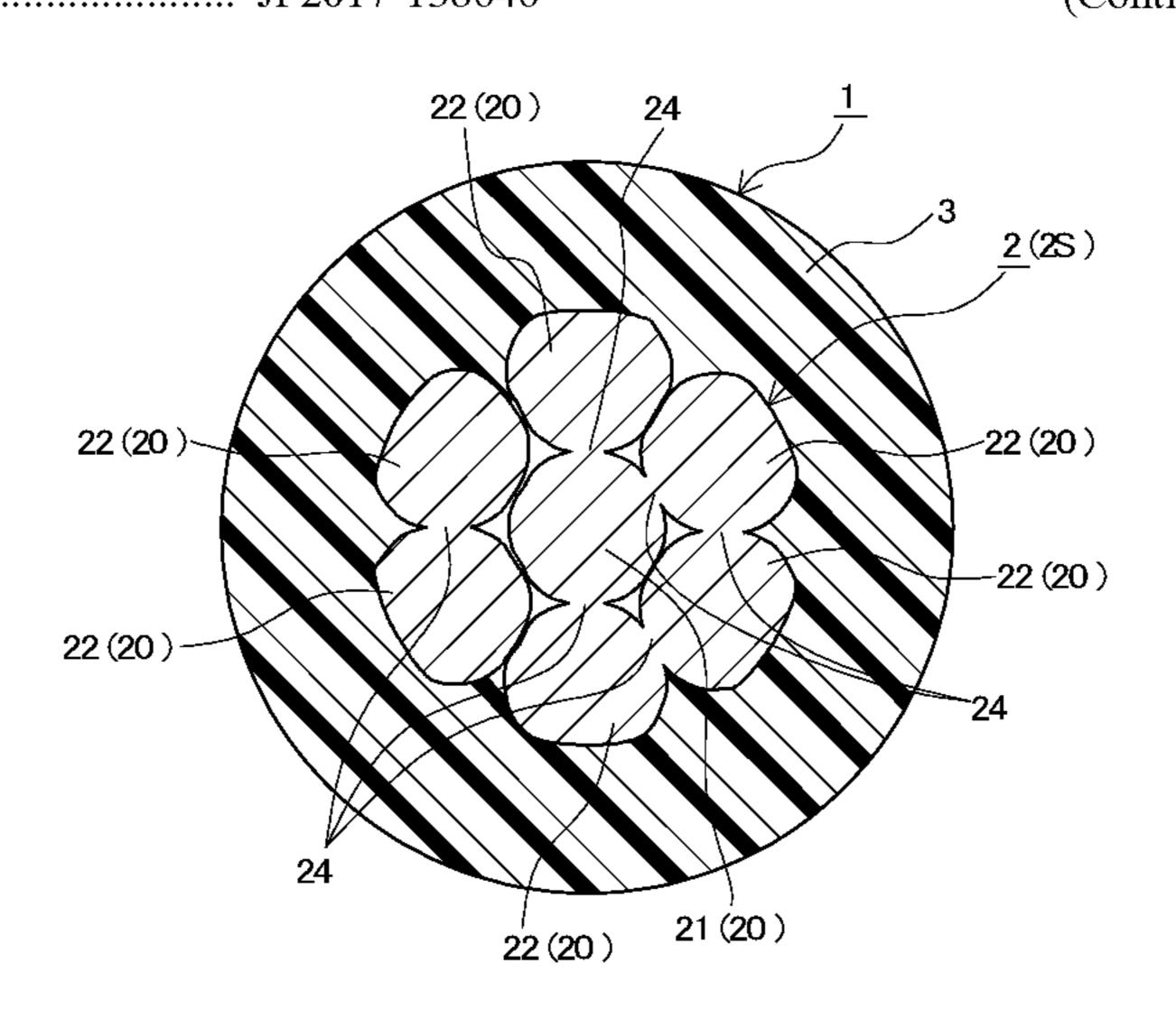
by twisting together a plurality of elemental wires constituted by copper or a copper alloy, and the covered electrical wire includes a metallically bonded portion where the elemental wires that are adjacent to each other are metallically bonded to each other.
