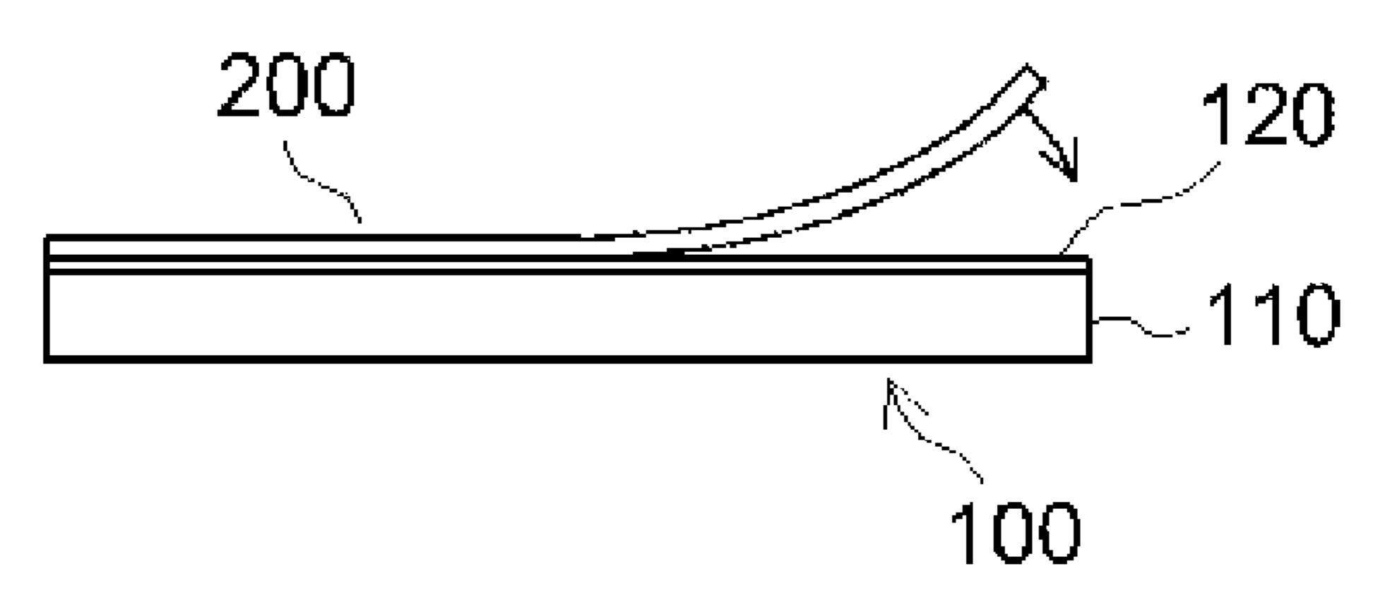
vided to at least one face of the waterproof layer. The PSA layer has a surface hardness of 0.5 MPa or less.
