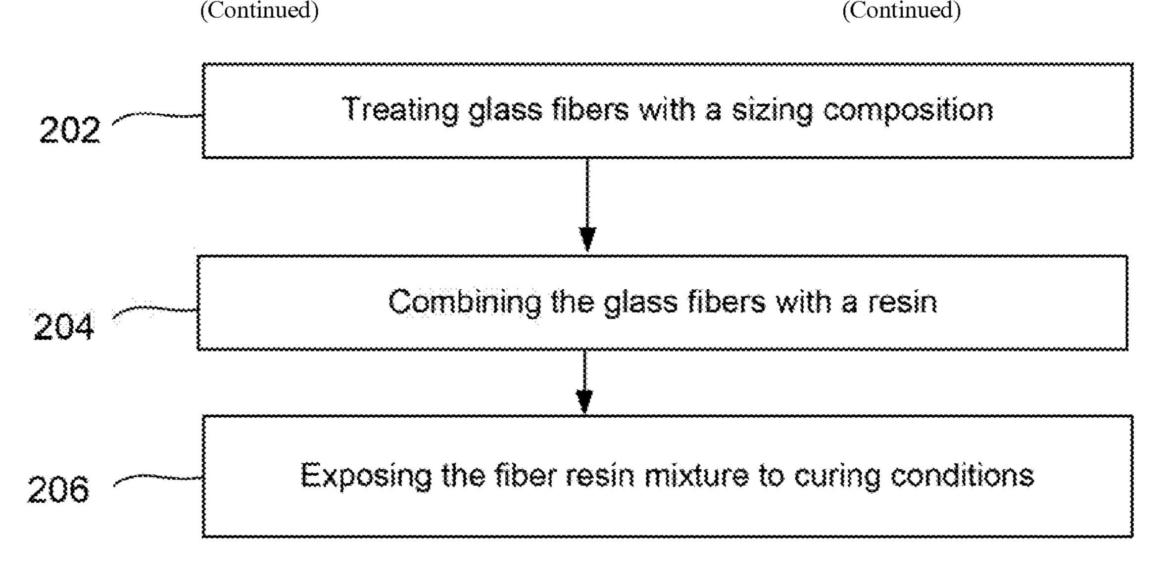
may then be cured so that the monomer polymerizes to form a thermoplastic polymer matrix of the fiber-reinforced composite. The thermoplastic polymer matrix may be formed by in situ polymerization initiated from both the surface of the glass fibers and the resin. The fiber-reinforced composite formed may be at least 70 wt. % glass fiber.
