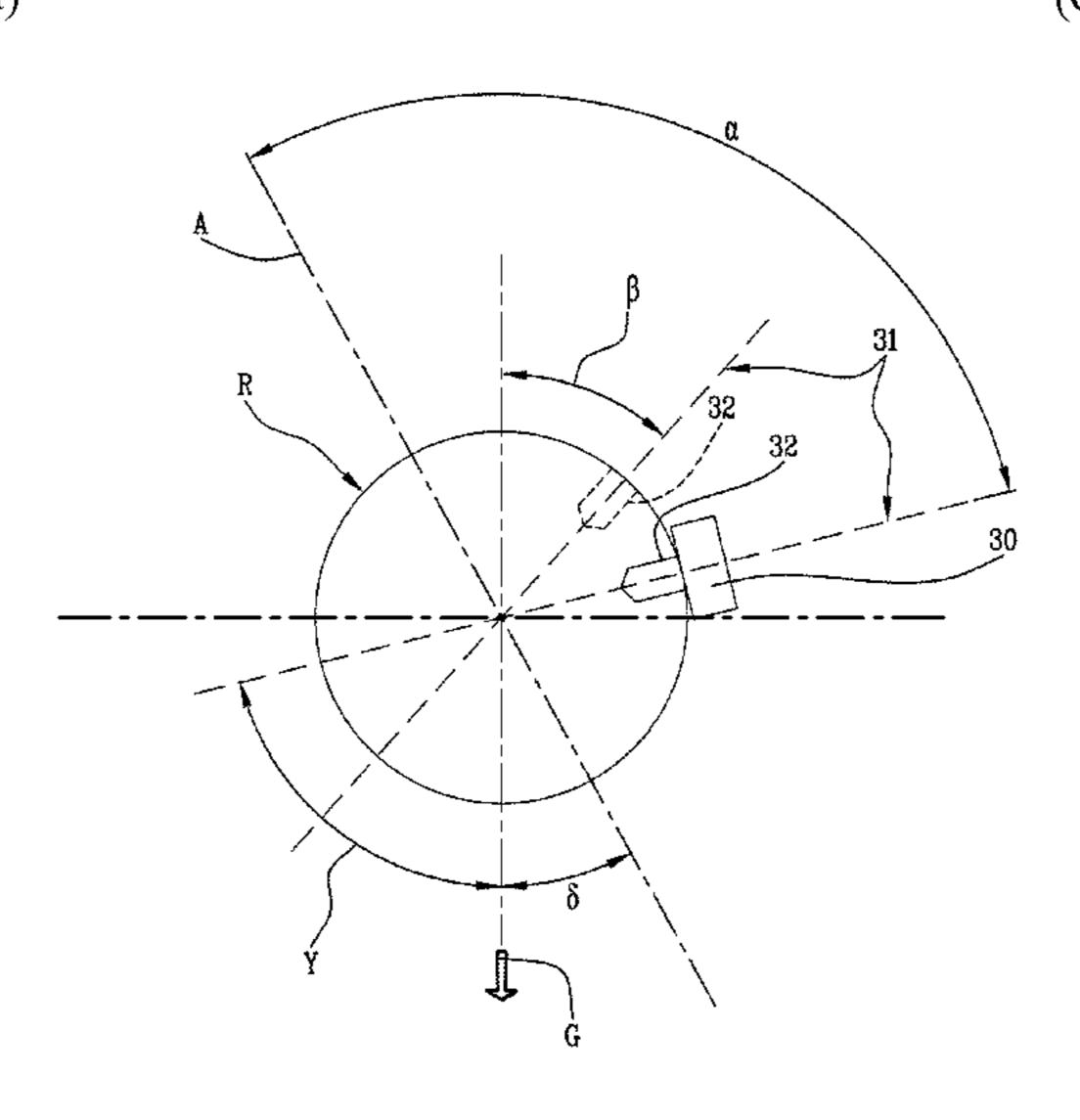
calculating and storing the angular displacement between the angular positions of the motor and the conveyor corresponding to the angular displacement between the zero reference and the force of gravity.
