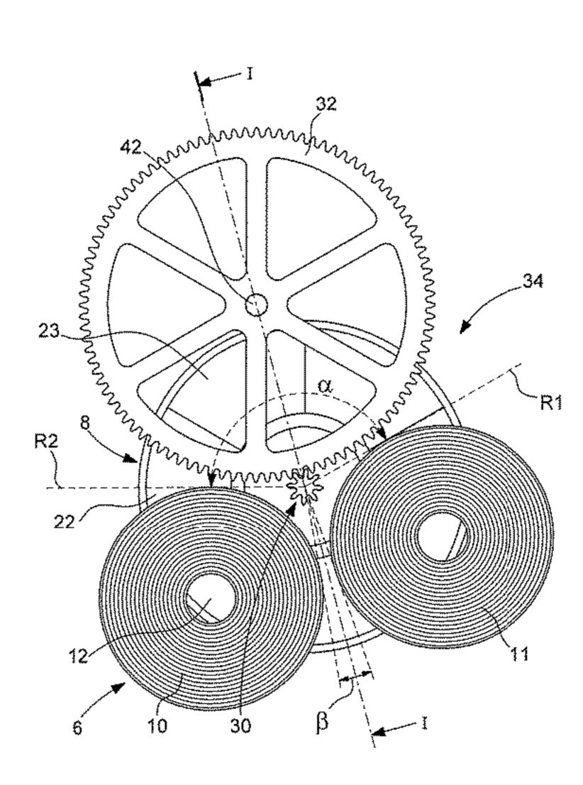
being partially arranged between the two magnetic plates, in an angular sector of the circular space that is left free by the electromagnetic transducer, so as to engage with the pinion. Advantageously, said wheel has a roller that is almost or entirely non-conductive and a non-magnetic staff.
