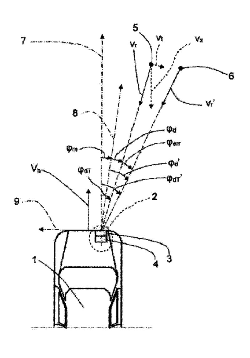
determine whether the radar detector (3) is misaligned based on the relation, where the total detection angle  $(\varphi_{dT}, \varphi_{dT}')$  equals the sum of a known mounting angle  $(\varphi_m)$  between the x-axis (7) and the radar detector's mounting direction (8), and a detection angle  $(\varphi_d, \varphi_d')$ . The present disclosure also relates to a corresponding method.
