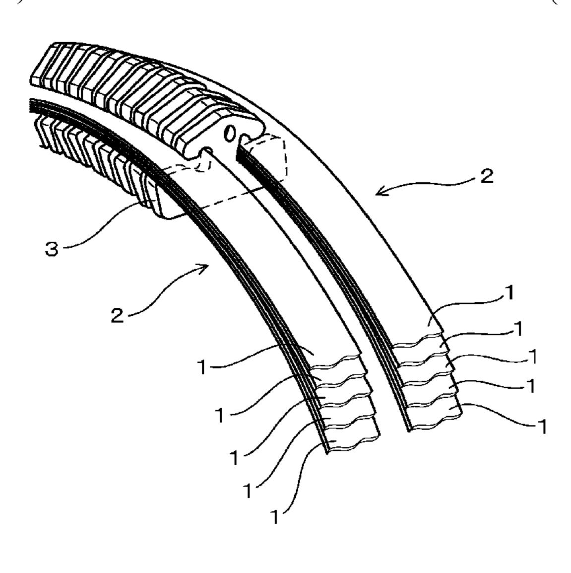
unavoidable impurities. The ring member has a tensile strength of 1,700 MPa or more. The nitrided layer has a surface hardness of HV800 to HV950.
