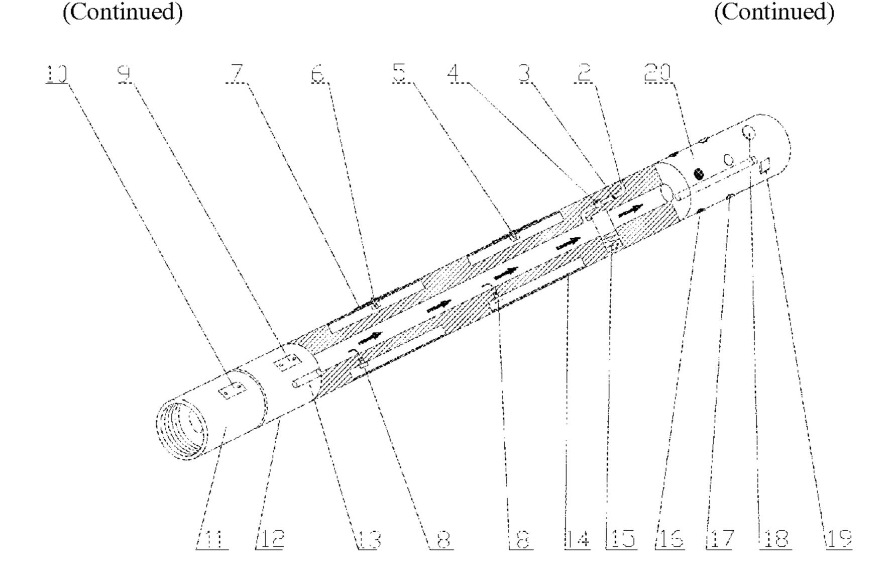
time gas parameter, lithologic and coal seam information, for on-site assessment of outburst risk. During drill bit replacement, gas pressure, temperature, flow velocity, wave velocity, electromagnetic radiation, and an acoustic signal are recorded in real time, to calculate stress of the coal seam and coal seam outburst risk. On-site measurement is done while drilling without sampling and can use multiple parameters to perform synchronous measurement to obtain a comprehensive evaluation.
