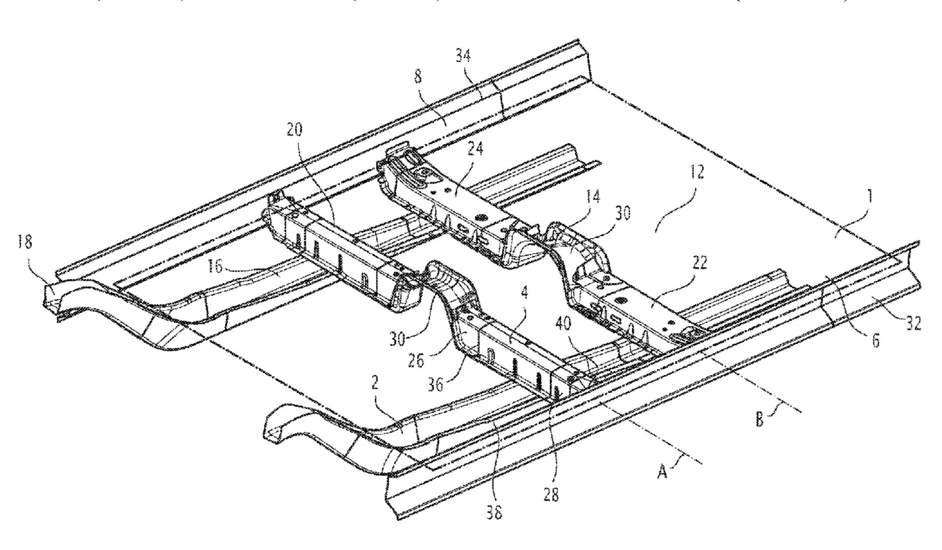
end, the resistance to plastic deformation of the central portion being greater than the resistance to plastic deformation of the end portion, and in that the intermediate part of the transversal beam extends upright of the longitudinal beam such that the end portion of the transversal beam extends transversally between the longitudinal beam and one of the sides of the floor panel.
