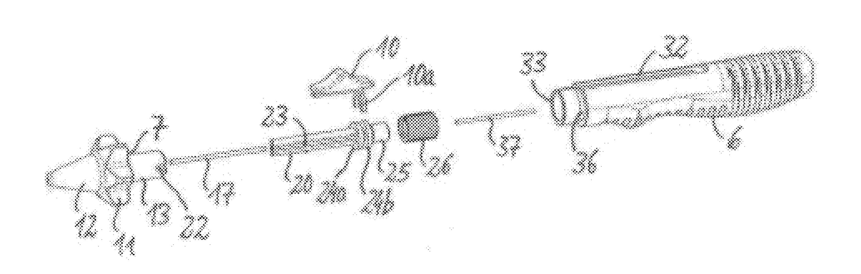
an eccentric axial wire passage opening. The two passage openings are arranged axially one behind the other and are in alignment in the wire release position and are out of alignment in the wire clamping position.
